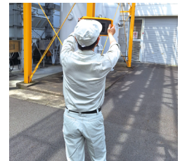
An employee checking for air leaks
